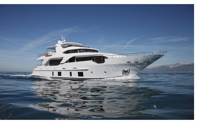
LOA: 93'6" (28.50m) BEAM: 23'1" (7.03m) DRAFT: 5'11" (1.81m) ENGINES: CAT C18 ACERT 747kW @ 2,300 rpm or MTU 8V2000 M72 720 kW @ 2,250 rpm (optiona) SPEED: 14/13 knots (max/cruising) RANGE: 1,500 nm @ 10 knots CONSTRUCTION: composite EXTERIOR DESIGN: Stefano Righini INTERIOR DESIGN: Carlo Galeazzi
